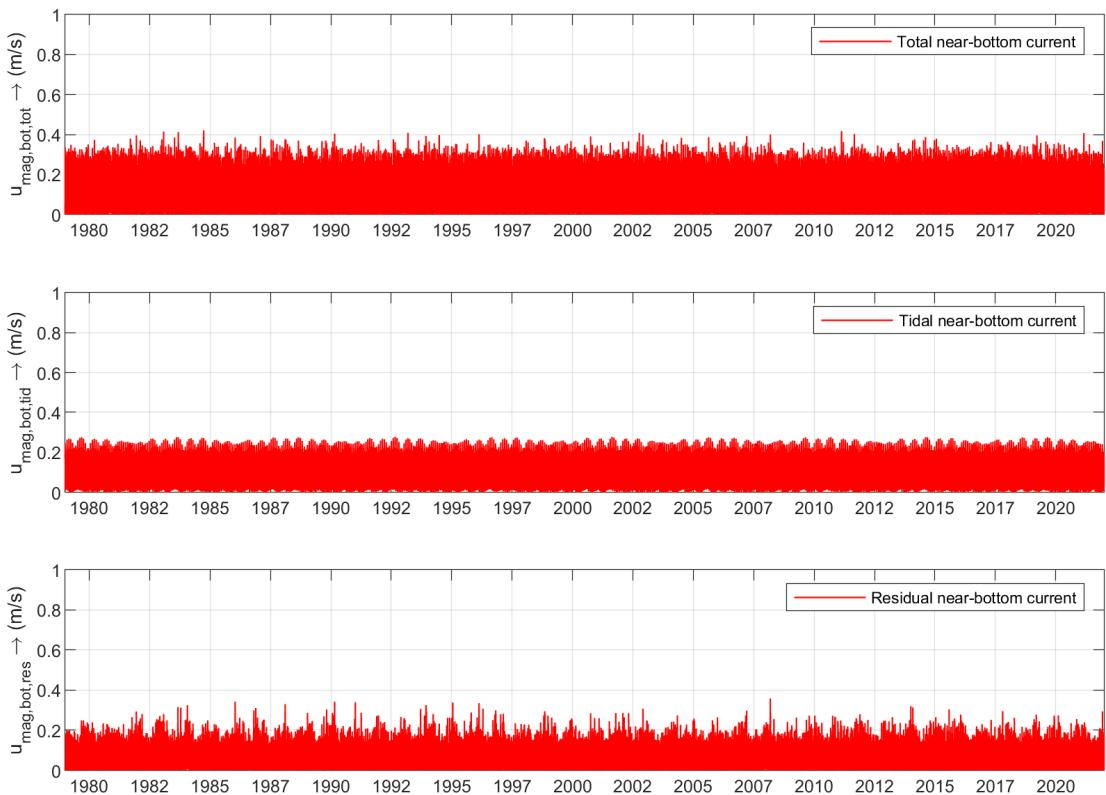
Figure 3.20 Timeseries of total, tidal and residual near-bottom current velocities at WTG11.
