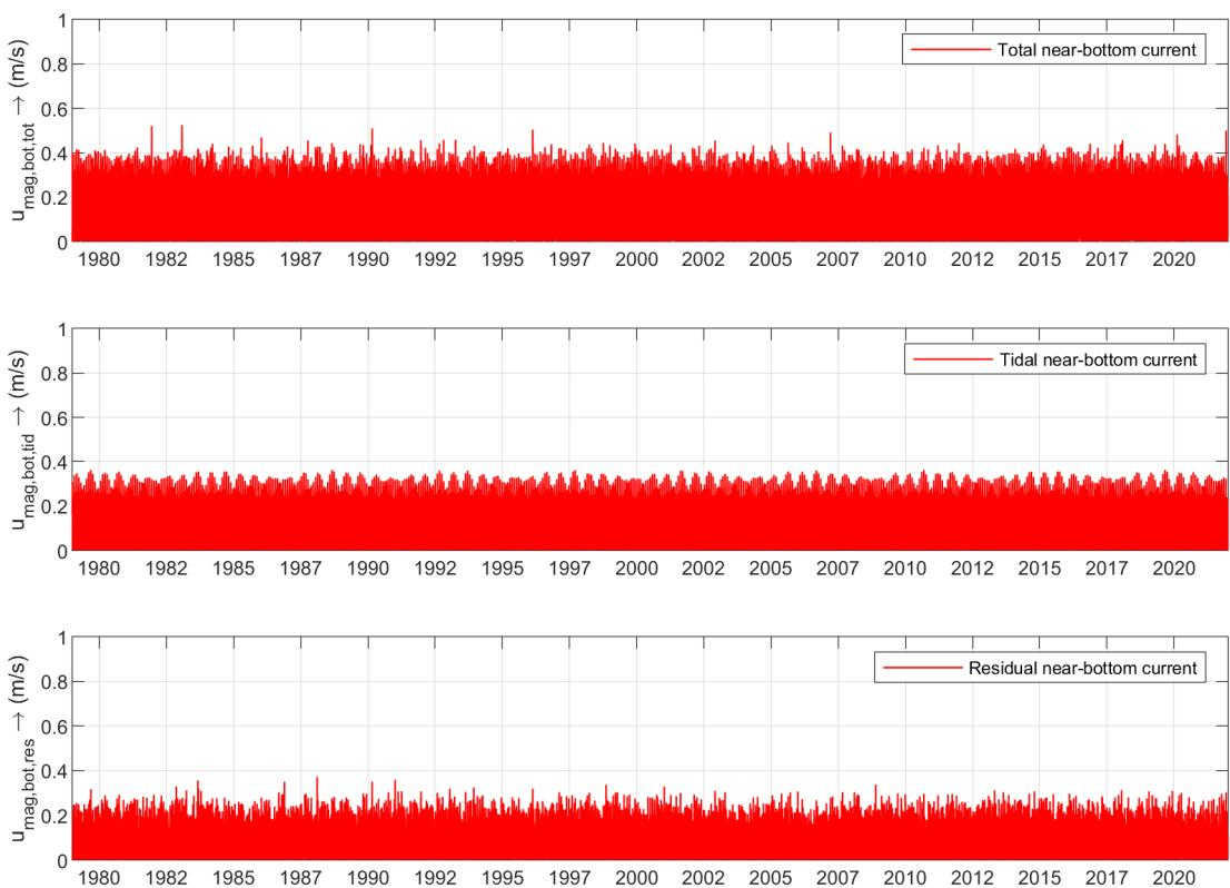
Figure 3.14 Timeseries of total, tidal and residual near-bottom current velocities at WTG15.
